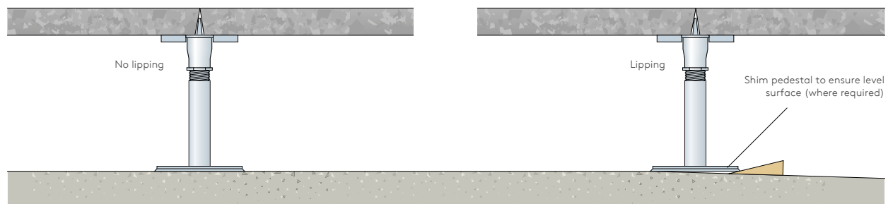
Figure 6. Correcting a panel lipping condition.
