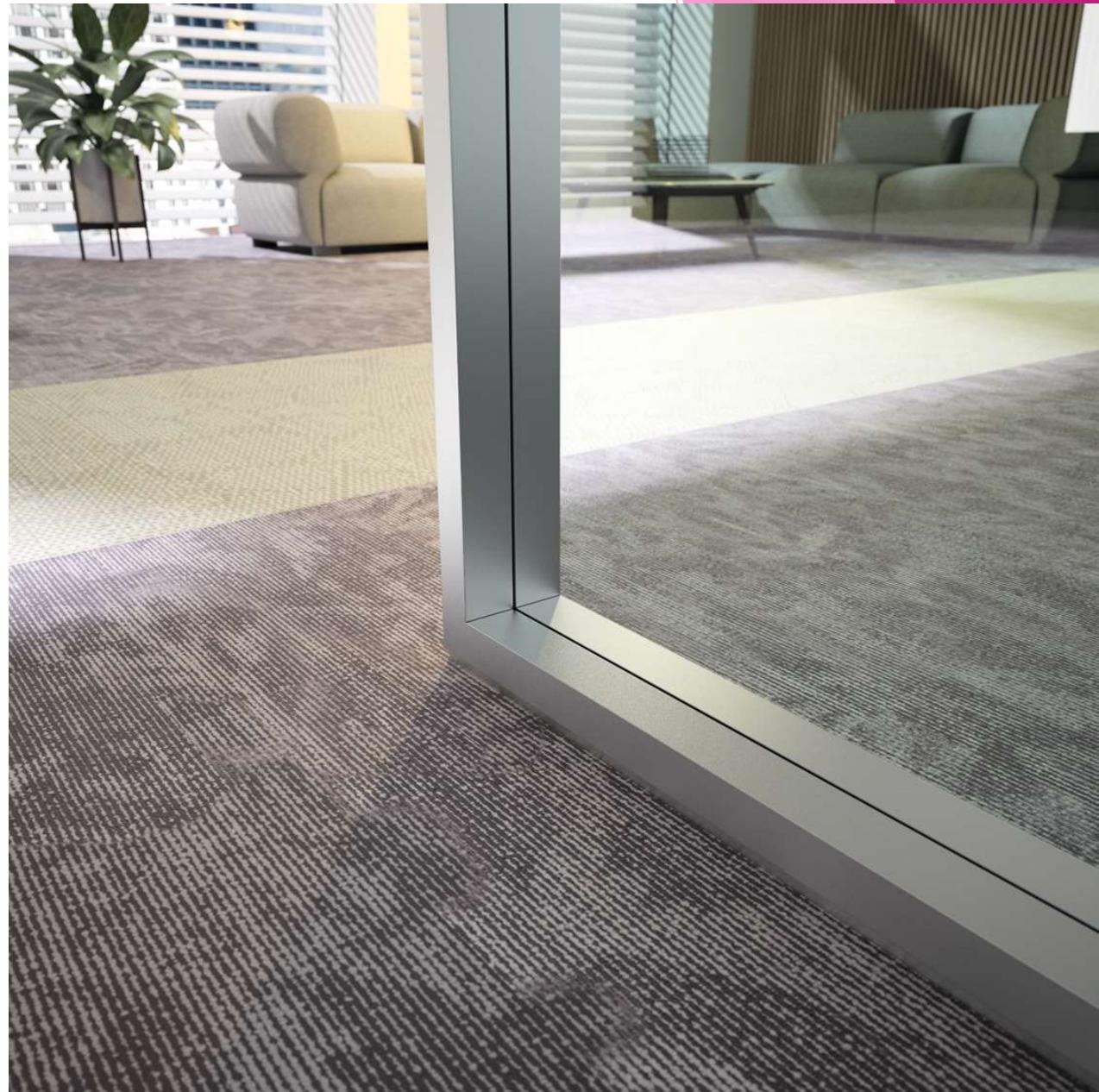
Single glass removable partition, made of extruded aluminum structure with 10mm to 16mm colorless laminated glass panels, glued together by a transparent 4mm polycarbonate profile.
